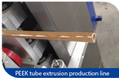
PEEK tube extrusion production line
