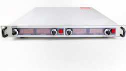
Wisman's MSC 2-channel output high-voltage power supply system. Each channel can be used and controlled by MSC system independently via front panel, providing with voltage and current monitor on the front panel. These MSC systems are specifically designed with proprietary linear power conversion techniques to provide exceptionally low ripple and noise. MSA system can be controlled remotely, with RS-485 interface, overcurrent, arcing and short circuit protection options.
