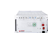
Wisman's AML series is a high-voltage power amplifier for industrial and research applications. The unique all-solid-state high-voltage insulation design can achieve high conversion rate, wide bandwidth and low noise operation. The four-quadrant active output sinks or outputs current to reactive or resistive loads within the entire output voltage range. This type of output is essential for achieving accurate output response and the high slew rate required for various loads, such as high capacitive or reactive loads. The amplifier is a non-inverting amplifier.
