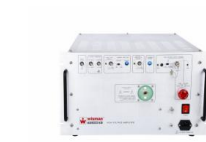
Wisman's AMK series is a high-voltage power amplifier for industrial and research applications. The unique all-solid-state high-voltage insulation design can achieve high conversion rate, wide bandwidth and low noise operation. The four-quadrant active output sinks or outputs current to reactive or resistive loads within the entire output voltage range. This type of output is essential for achieving accurate output response and the high slew rate required for various loads, such as high capacitive or reactive loads. The amplifier is a non-inverting amplifier.
