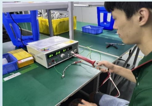
High voltage test
